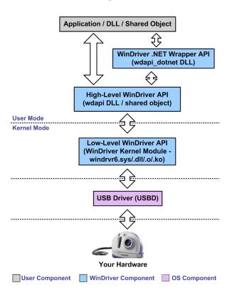
The device driver developed with WinDriver (yourapp.exe/dll/so) accesses hardware through the WinDriver kernel module (windrvr1460.sys/ko) using WinDriver's API functions.
